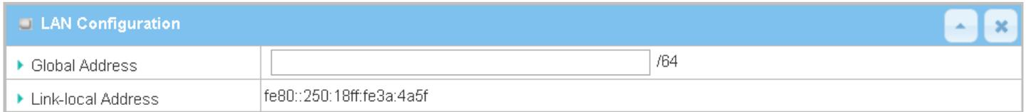
The screenshot shows a window titled "LAN Configuration" with a blue header bar. Below the header, there are two rows of configuration items. The first row is "Global Address" with an empty text input field followed by "/64". The second row is "Link-local Address" with the value "fe80::250:18ff:fe3a:4a5f".
