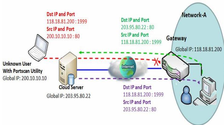
As shown in the diagram, Gateway has the IP address of 118.18.81.200 for WAN interface and 192.168.1.253 for LAN interface. It serves as a NAT gateway. Users in Network-A initiate to access cloud server through the gateway. Sometimes, unknown users will simulate the packets but use different source IP to masquerade. With the SPI feature been enabled at the gateway, it will block such packets from unknown users.
