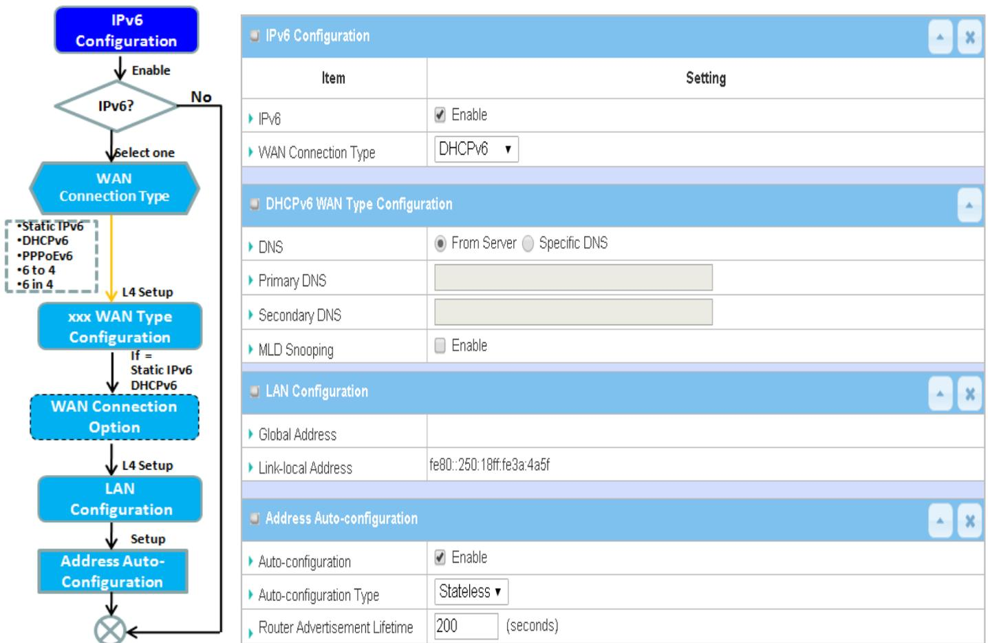
The **IPv6 Configuration** setting allows user to set the IPv6 connection type to access the IPv6 network. This gateway supports various types of IPv6 connection, including **Static IPv6**, **DHCPv6**, and **PPPoEv6**
