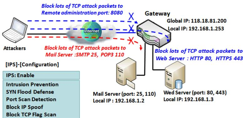
As shown in the diagram, the gateway serves as an E-mail server, Web Server and also provides TCP port 8080 for remote administration. So, remote users or unknown users can request those services from Internet. With IPS enabled, the gateway can detect incoming attack packets, including the TCP ports (25, 80, 110, 443 and 8080) with services. It will block the attack packets and let the normal access to pass through the gateway
