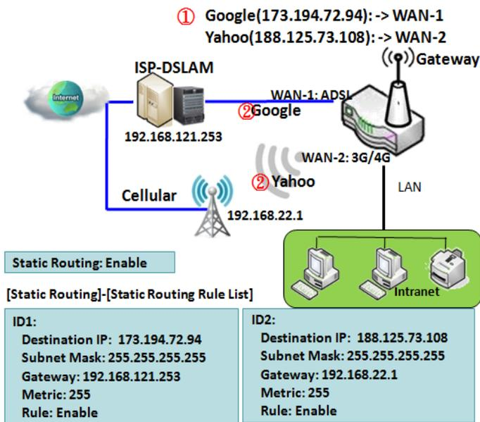
When the administrator of the gateway wants to specify what kinds of packets to be transferred via which gateway interface and which peer gateway to their destination. It can be carried out by the "Static Routing" feature. Dedicated packet flows from the Intranet will be routed to their destination via the pre-defined peer gateway and corresponding gateway interface that are defined in the system routing table by manual.
