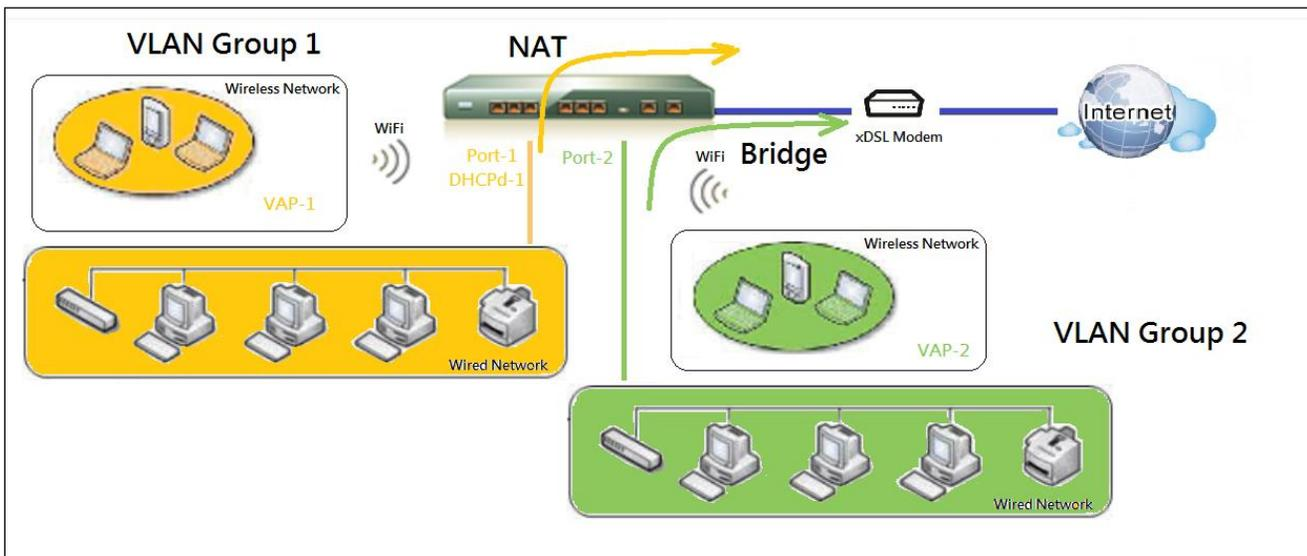
A port-based VLAN is a group of ports on an Ethernet or Virtual APs of Wired or Wireless Gateway that form a logical LAN segment. Following is an example.
