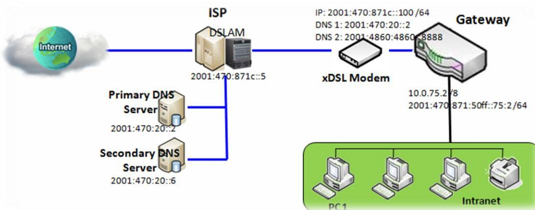
Above diagram depicts the IPv6 IP addressing, type in the information provided by your ISP to setup the IPv6 network.
