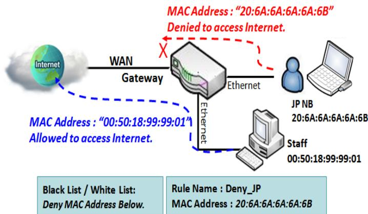
As shown in the diagram, enable the MAC control function and specify the "MAC Control Rule List" is a black list, and configure one MAC control rule for the gateway to deny the connection request from the "JP NB" with its own MAC address 20:6A:6A:6A:6A:6B.
