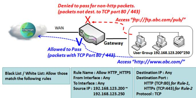
As shown in the diagram, specify "Packet Filter Rule List" as white list (Allow those match the following rules) and define the rules. Rule-1 is to allow HTTP packets to pass, and Rule-2 is to allow HTTPS packets to pass.
