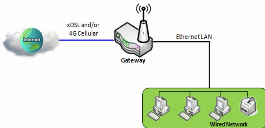
The Local Area Network (LAN) can be used to share data or files among computers attached to a network. Following diagram illustrates the network that wired and interconnects computers.
