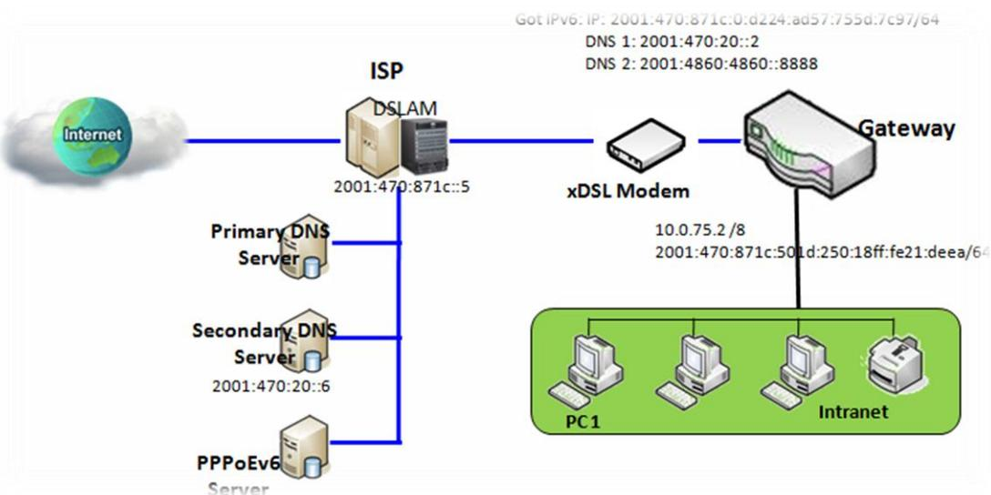
Above diagram depicts DHCP IPv6 IP addressing, the DHCPv6 server on the ISP side assigns IPv6 address, IPv6 default gateway address, and IPv6 DNS to client host's automatically.
