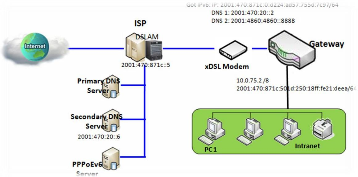
The diagram above depicts the IPv6 addressing through PPPoE, PPPoEv6 server (DSLAM) on the ISP side provides IPv6 configuration upon receiving PPPoEv6 client request. When PPPoEv6 server gets client request and successfully authenticates it, the server sends IP address, DNS server addresses and other required parameters to automatically configure the client.
