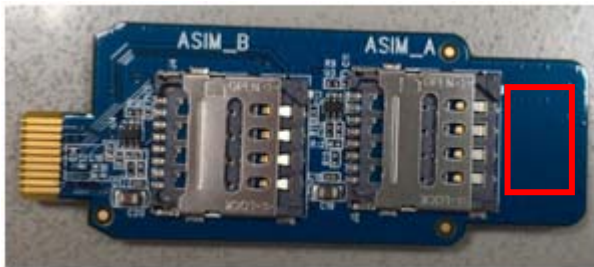
Bottom View (SIM slots for 3G/4G module)
