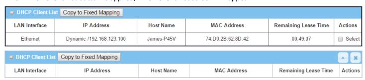
When the DHCP Client is selected and **Copy to Fixed Mapping** button is applied. The IP and MAC address of DHCP Client will apply to the Mapping Rule List on specific DHCP Server automatically.
